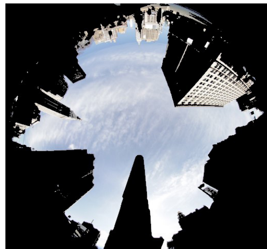
Segmentation result (the non sky region is colored in black) obtained applying an original segmentation method developed in our research team.
